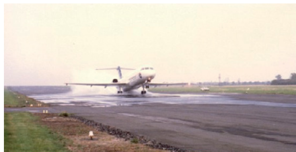
Water Ingestion Trials met de Fokker 100 te Cranfield, U.K.
